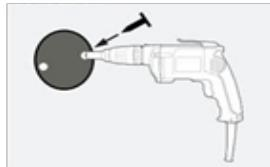
Place the plastic wall plugs in the holes then insert the screws leaving part of the screw out of the wall to grip to the Decoy Dome Camera. Then, place the camera over the screws and slide to the right to fix it to the wall.
